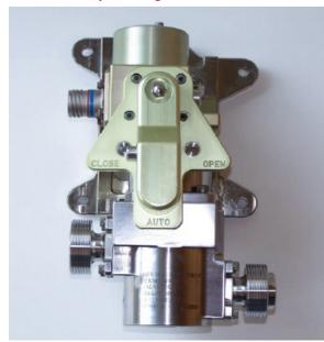
Part number 12085-5 is used on the International Space Station in the Hydrogen Vent Assembly and Major Constituent Analyzer in the Environmental Control and Life Support System. The valve is totally pressure balanced using edge welded Inconel bellows. Photo from: valvetech.net
