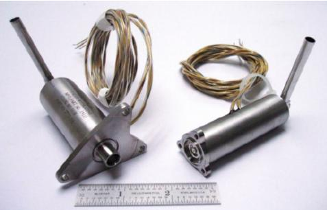
ValveTech has qualified and flown a number of propellant control valves for small, monopropellant rocket engines in the 0.1 to 5.0 LBf. range. The valve design uses an AF-E-411 elastomeric puck for exceptional sealing capability.
